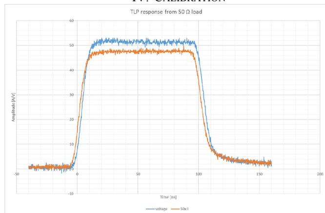
Figure 4 – Uncorrected pulse responses of a 50 • resistor
