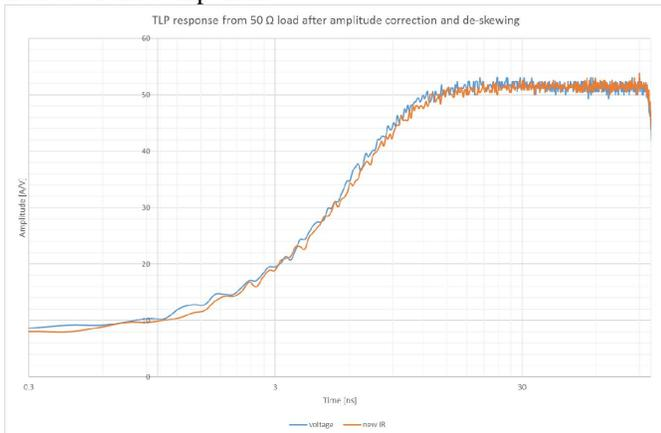
Figure 6 – Corrected pulse responses on a log-time scale
