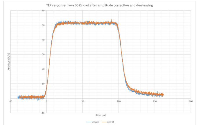
Figure 5 – Corrected pulse responses of a 50 • resistor
