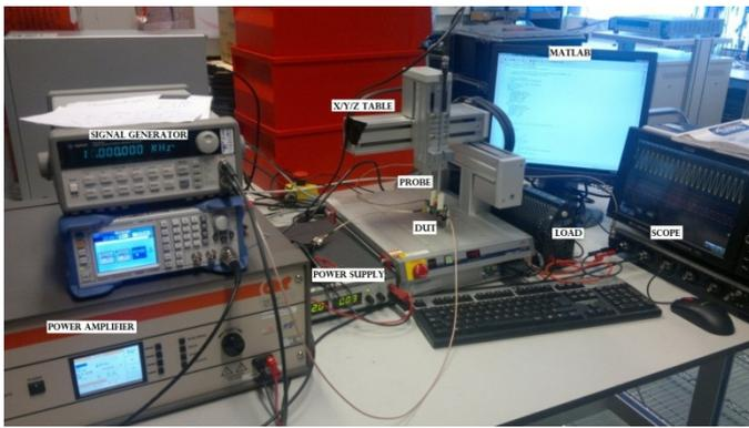
Figure 7 - Total LF H-field immunity test system
