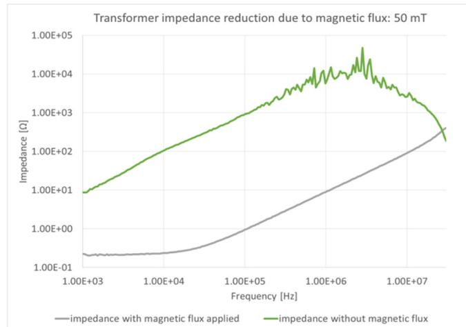
Figure 1 - Transformer inductance degradation due to magnetic flux
