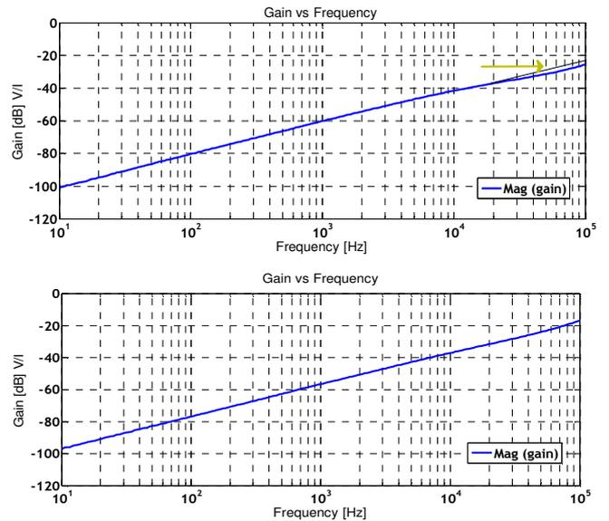
Figure 4 – Calculated transfer function versus measured transfer function. a) Wide strip b) Thin wire
