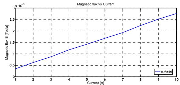
Figure 5 - Injection probe linearity
