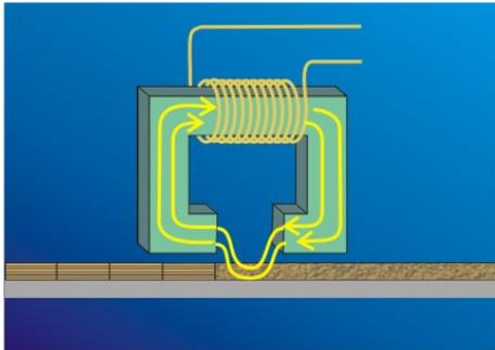
Figure 2 - Recording head magnetic flux
