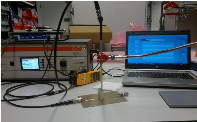
Figure 3 - H-field injection probe over a micro-strip test board
