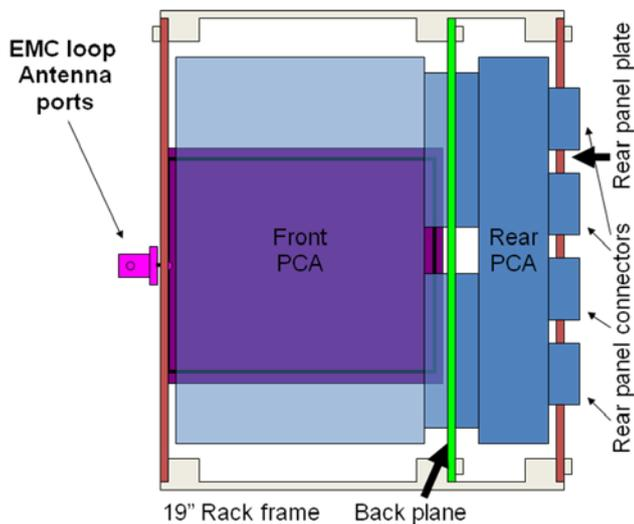
Figure 3 - Side view for low frequency radiated EMC testing in a rack
