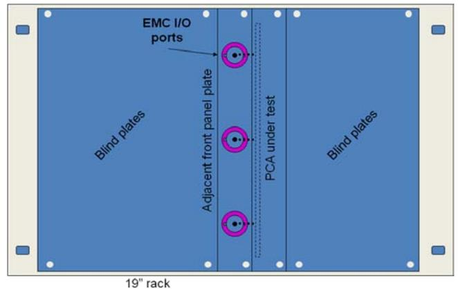
Figure 2 - Front view for conducted EMC testing in a rack
