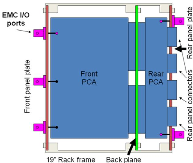
Figure 1 - Side view for conducted EMC testing in a rack
