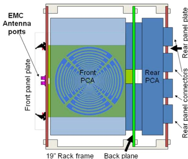
Figure 4 - Side view for RF radiated EMC testing in a rack
